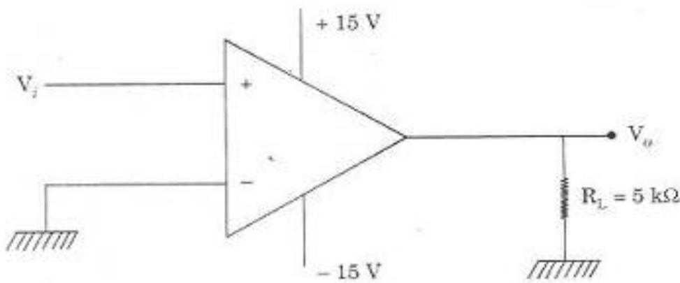
If  $V_i$  is a sinusoidal input, its value for which the comparator saturates is :
