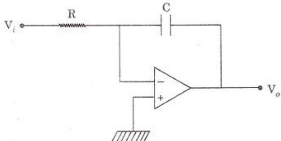
If  $V_i$  is a step voltage having levels 0 V and +5 V, the rate of change of output voltage is :
