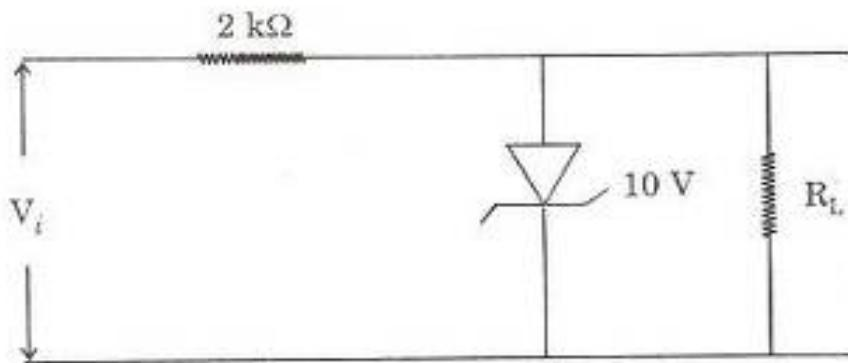
If  $V_i$  changes from  $25 \text{ V}$  to  $50 \text{ V}$ , the change in the current through Zener is :
