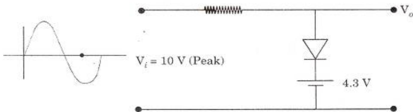
If the junction barrier voltage is 0.7 V, the output waveform will be :
