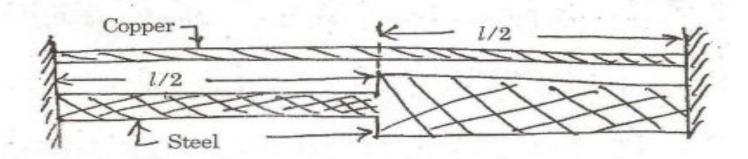
Cross-sectional area of copper bar =  $\mathrm{Am^2}$  throughout. Cross-sectional area of steel bar =  $\mathrm{Am^2}$  and  $\mathrm{2A^2}$  for each half of the length (as shown above). Co-efficients of expansion of copper and steel are  $\alpha$  and 1.3 $\alpha$ , while elastic moduli for these materials are E and 0.5 E respectively. Find the stresses induced in the bars due to rise ( $t^{\circ}\mathrm{C}$ ) of temperature.
