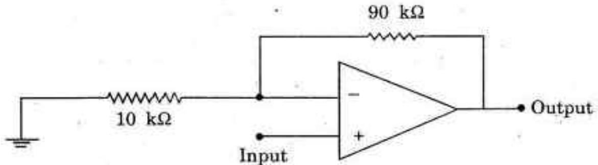
The closed loop gain of the amplifier is :
